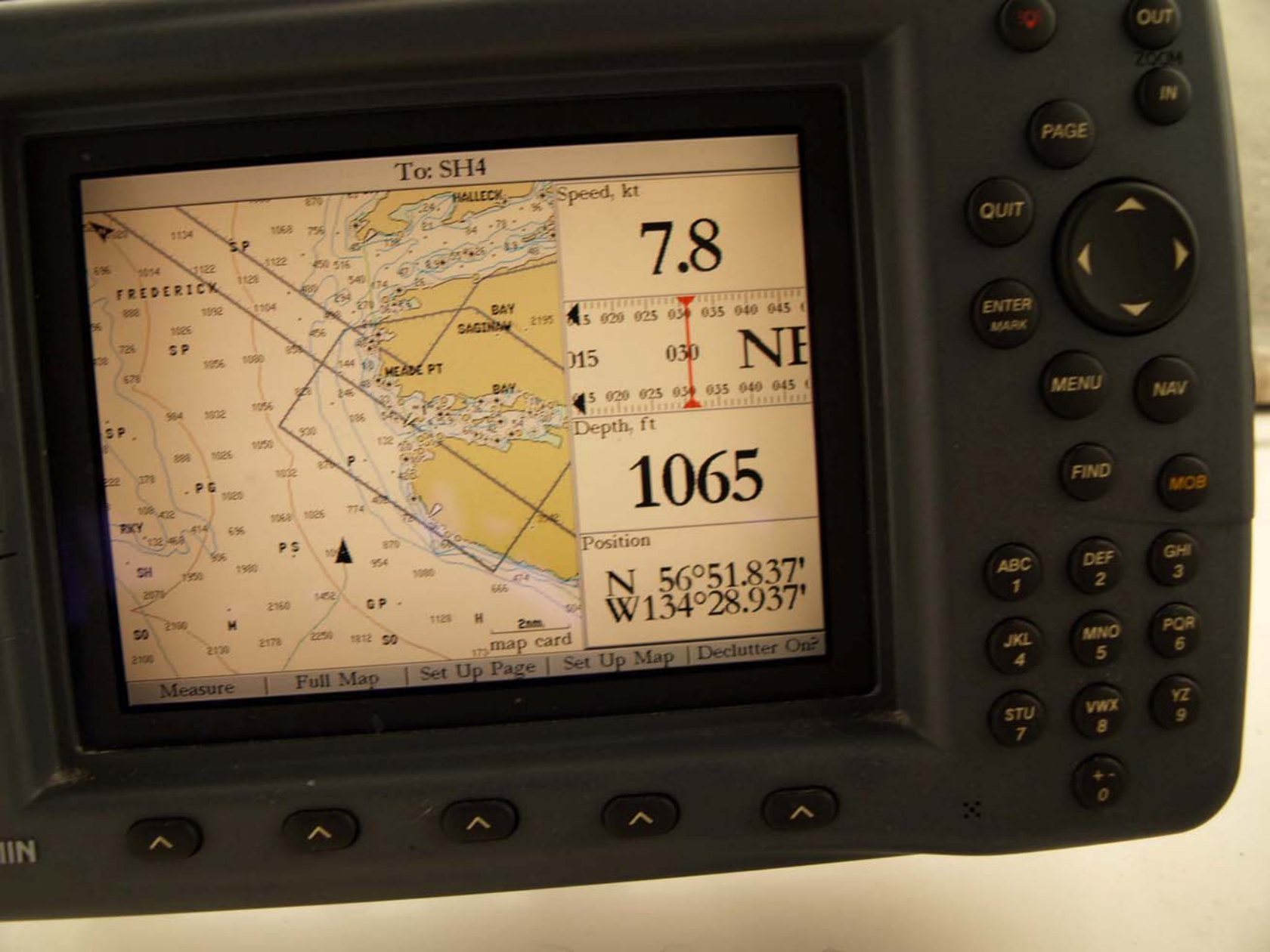
Used GPS everywhere we went...both boats. In this mode, it gave speed, bearing, water depth, and location in lat/long.
